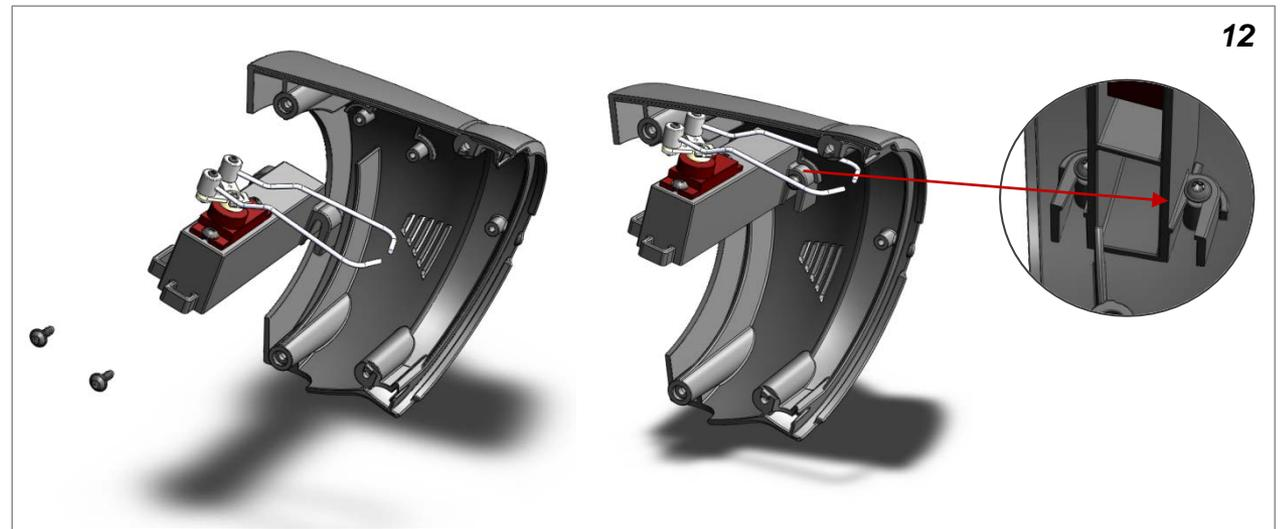
Insert servo assembly into left main housing and secure with 2 screws
